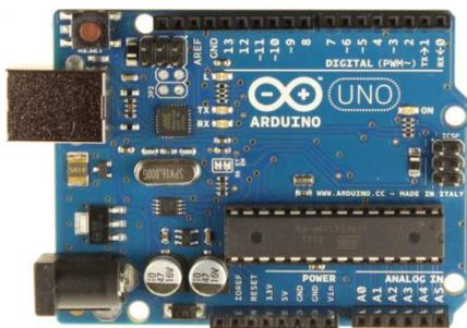
Gambar 2.1 Board Arduino Uno [2]
