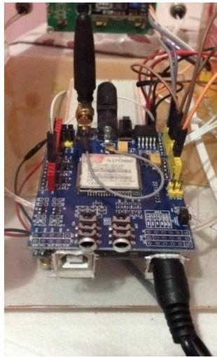
Gambar 4.4 SMS Gateway Icoms SIM900
