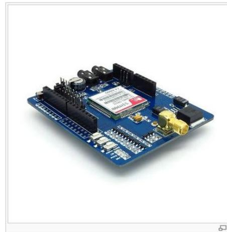
Gambar 2.2 SIM900 GSM GPRS Shield Module [3]
