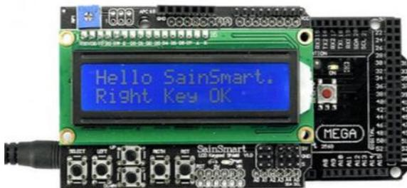
Gambar 2.5 LCD Display 1602 [6]
